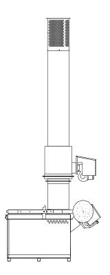
■ Concave refractory bottom specifically designed to insure burnout and total destruction of solid and liquid wastes.
